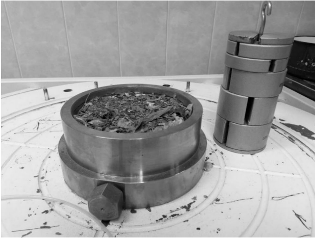
Fig. 4 Dry specimen installed in the oedometer cell and weight used for initial compaction
