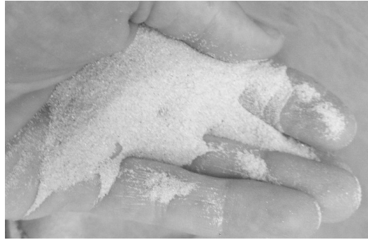
Figure 5. Tested sand sample with fraction size in a range from 0 to 1 mm.
