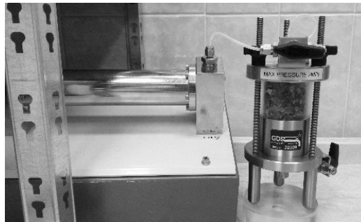
Figure 4. The advanced pressure/volume controller piston—pressure chamber; the GDS toxic-cell—sample chamber.
