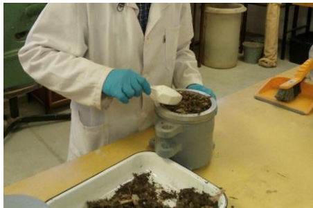
Figure 5. Filling the mould with waste sample.
