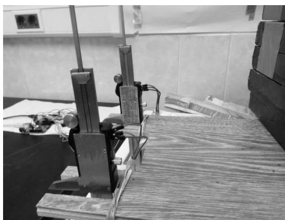
Figure 2 Two callipers connected with Arduino Uno
