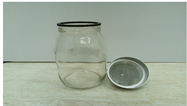
Figure 3. Large water pycnometer (1dm 3 volume) with aluminum screen for the light mass components
